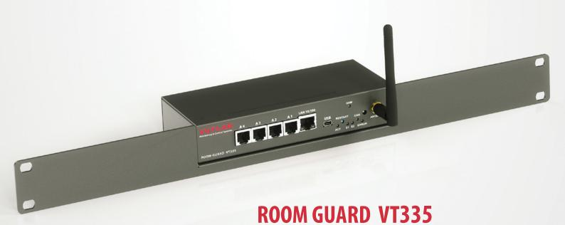
Environmental monitoring of any facilities, control of security breaches, temperatures, smoke, water leakages, voltages and more.
